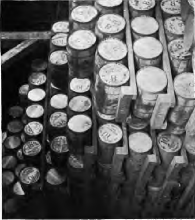
Fig. 2. Skids for piling Heavy Kegs.*
